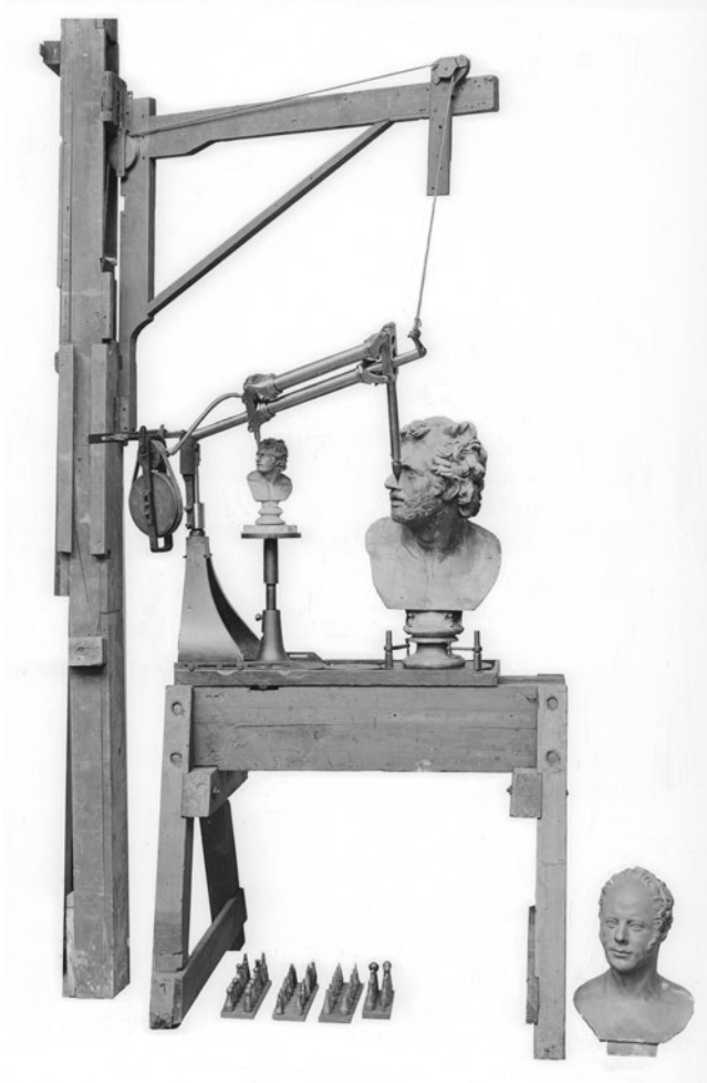
Benjamin Cheverton's machine to copy sculptures, based on a design by James Watt
